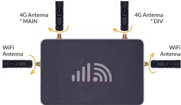
When installing the antennas, put the router and antennas in a straight direction to avoid bending the pins. Twist the SMA-male connector on the antennas in the clockwise direction to install the antennas on the router.
